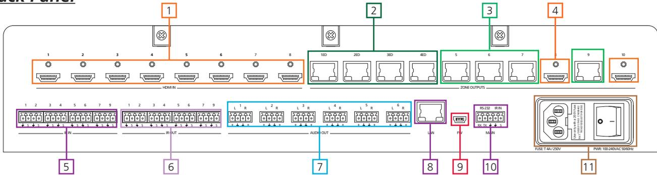
1. HDMI Input - Connect HDMI sources to these ports
