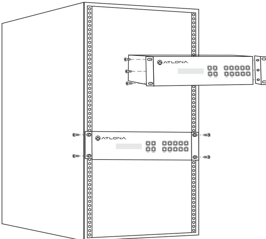
To rack mount the UHD-PRO3-88M unit: use the rack mount ears, the 6 screws from the sides of the UHD-PRO3-88M, and 4 rack screws.
