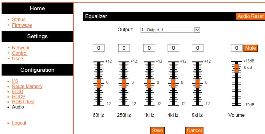
The audio page supports adjustment of 5 band EQ for the analog audio outputs ensuring the best audio performance for each zone. 5 band frequency options at 63Hz, 250Hz, 1kHz, 4kHz, and 8kHz as well as zone output volume and mute.
