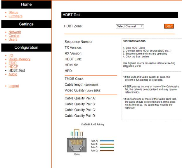
The HDBT page provides testing of Ethernet cables connected to the HDBaseT port on the matrix. To perform an HDBaseT test, do the following:
