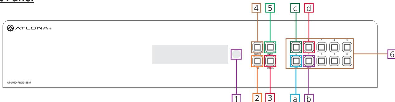
1. IR Receiver Window - Receives the signal from the included IR Hand Held Remote Control or 3rd party controller
