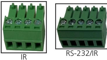
Two types of female captive screw connectors have been included: 4 pin (IR) and 5 pin (RS-232/IR).
