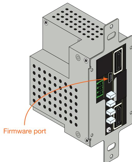
3. Connect the USB-A to USB mini-B cable between the PC and the firmware port on the AT-HDVS-210H-TX-WP. The unit will be powered by the USB cable.
