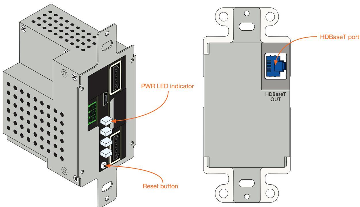
3. Press and hold the **Reset** button for approximately 5 seconds. Release the **Reset** button once the **PWR** LED indicator begins to flash. The number of flashes will indicate the currently selected IP mode.
