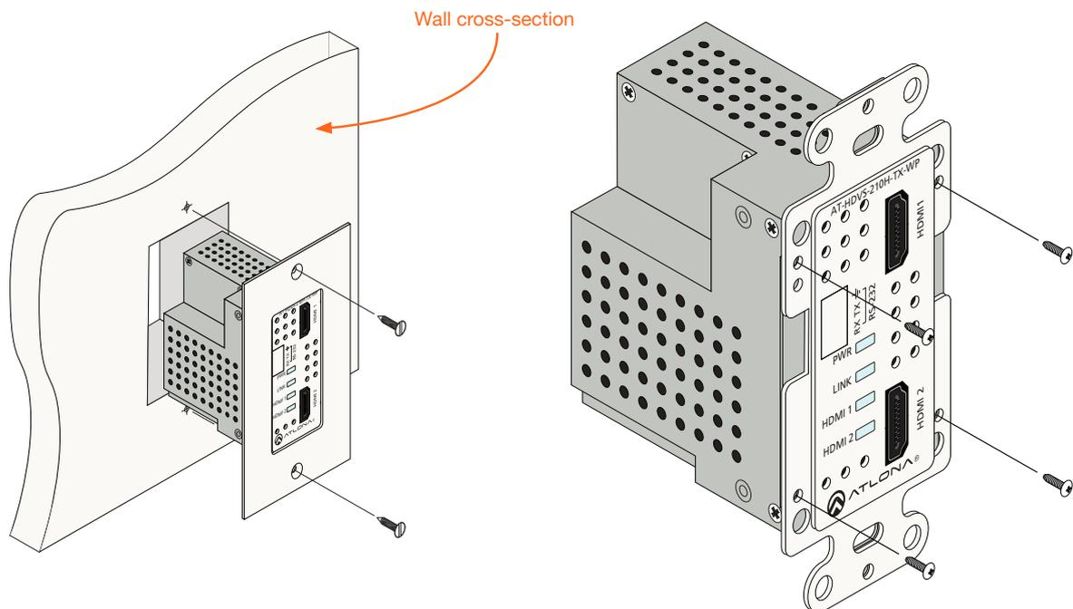
2. Remove the four screws, holding the faceplate to the assembly, using a Phillips screwdriver. Once the screws are removed, gently remove the faceplate by pulling it toward you.
