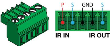
**IR IN** is connected by a power, ground, and signal wire. Use a 12V IR receiver with it (e.g. AT-IR-CS-RX purchasable through [atlona.com](http://atlona.com)).
