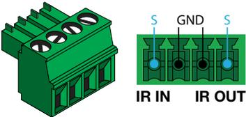
**IR IN** is connected by a ground and signal wire. Use with 3rd party control systems. For easy termination, Atlona recommends using the 2 meter IR cable AT-LC-CS-IR-2M (purchasable through [atlona.com](http://atlona.com)).
