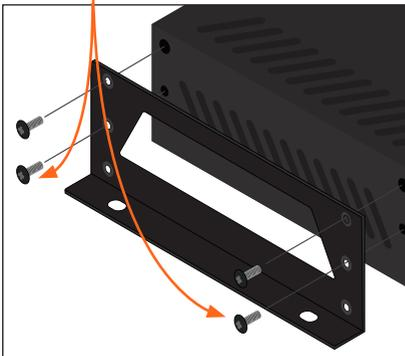
4. To provide added stability to the mounting bracket, use two of the included screws and attach them to the two holes, directly below the enclosure screws, as shown above.
