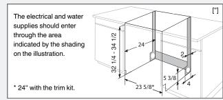
Make sure the area on which the dishwasher is to be installed is firm. Adjust the adjustable feet so that the dishwasher is level.
