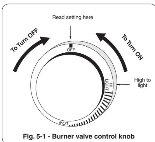
Fig. 5-1 - Burner valve control knob
