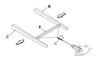
STEP 4: Using the Allen Key to tighten all bolts
