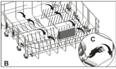
Bringing the tines to the horizontal position by holding them from the tips may cause them to bend. Therefore, it will be appropriate to bring the tines in the middle to horizontal or vertical position by holding them from their stems and pushing in the direction of arrow.
