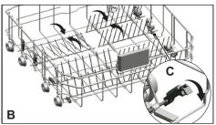
Bringing the tines to the horizontal position by holding them from the tips may cause them to bend. Therefore, it will be appropriate to bring the tines in the middle to horizontal or vertical position by holding them from their stems and pushing in the direction of arrow.
