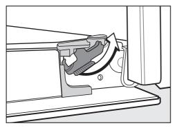
Release the locking clamps by turning them as far as they will go. You could damage the oven if you remove the door incorrectly. Do not pull the door horizontally off
