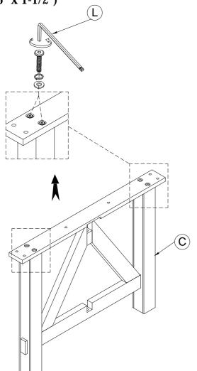
Step 2: Remove Leg stretcher (Bolts Ø5/16" x 3-1/8")
