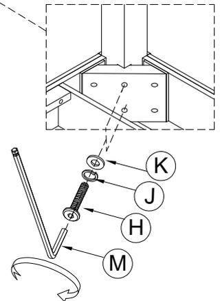
Step 5: Use the Allen Key to tighten all bolts
