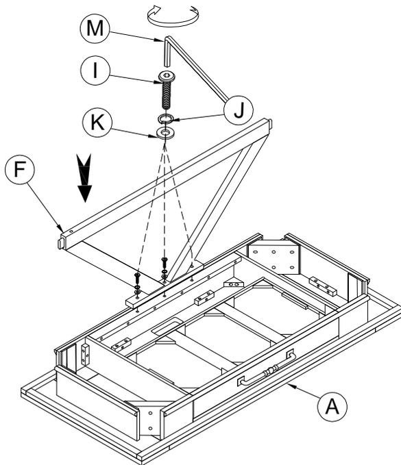
**Step 2: Use the Allen Key to tighten all the bolts**
