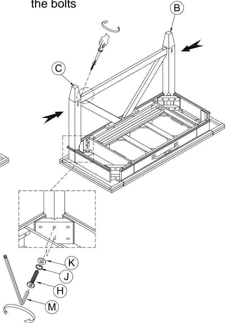
Step 3 & 4: Use a Phillips Head screw driver to tighten all screws
