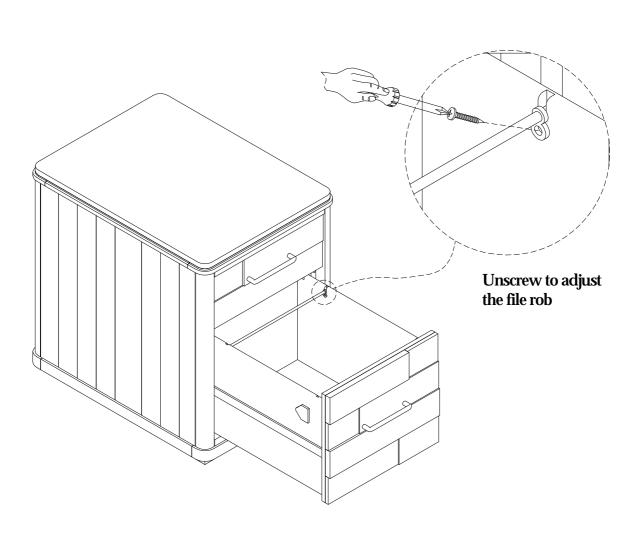
This furniture is equipped with safety hardware to prevent both drawers from being opened at the same time to prevent the cabinet from tipping forward. Please do not try to override this feature and completely close one drawer before opening the other.
