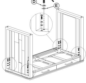
Step 2: Using the Allen key to tighten all bolts
