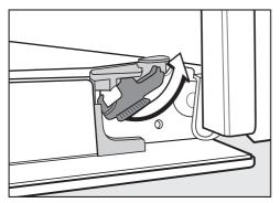
Release the locking clamps by turning them as far as they will go. Do not pull the door horizontally off its retainers, as they will spring back against the oven.
