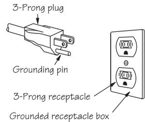
**⚠️ WARNING** Improper use of the grounding plug can result in a risk of electric shock. **Do not use an extension cord. If the power supply cord is too short, have a qualified electrician or servicetech install an outlet near the appliance.**
