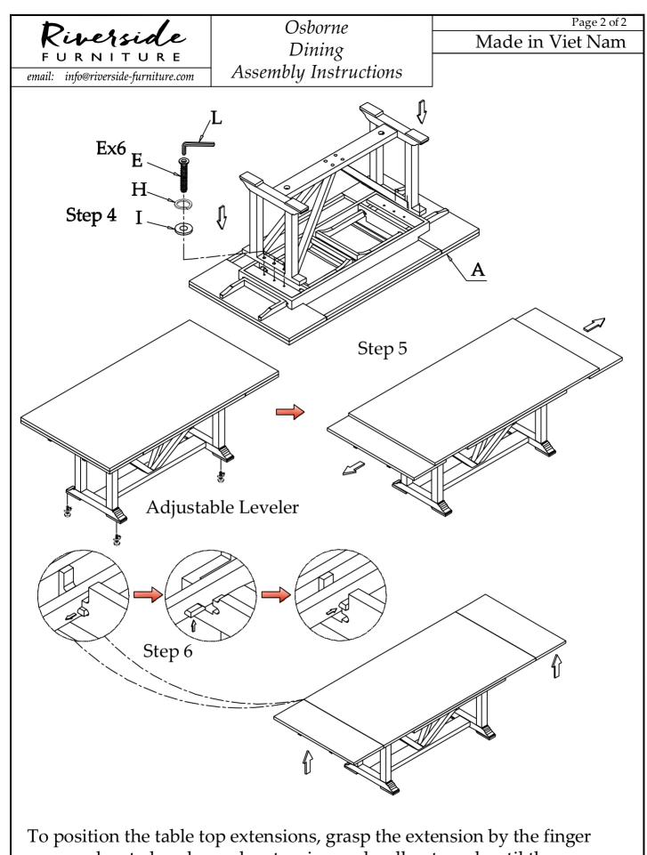
grooves located under each extension and pull outward until the extension stops, lift the extension upward until the top surfaces are level, push inward until there is no gap between the top and extension.
