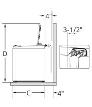
To ensure sufficient clearance for water lines and airflow, allow minimum clearances
