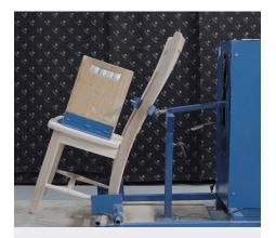
In the laboratory, a rocking motion is simulated for several hours to verify the chair's assembly strength and durability.
