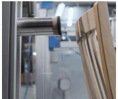
A chair falling on the floor, or being kicked, is also simulated using the hammer test. We repeat the operation several times and check for joint damage, cracks or breaks.
