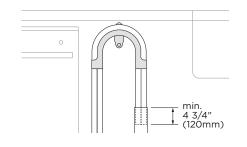
Pull both hoses through the support guide and rest in standpipe.
