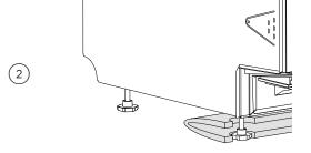
Gently tilt the DishDrawer™ Dishwasher back and align the seal to the front feet.
