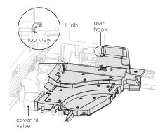
Position the cover fill valve into place before lowering the rest of the cover into position.
