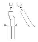
Thread wire clips onto the hoses before fitting them to the hose joiner. Secure using the wire clips. Fit the joiner to the Air Gap Kit and secure using the hose clamp. Ensure hoses are routed straight to the joiner, removing excess drain hose if necessary.
