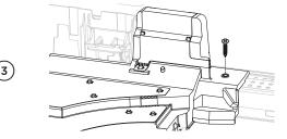
Remove the screw securing the cover. Set aside.
