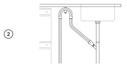
Pull both hoses through the drain hose support before threading the wire clips on to the hoses and fitting to the supplied hose joiner. Secure using the wire clips.
