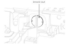
Fit a suitable cable clamp for the conduit through the metal knockout. Route wiring behind the tab and through the toroid removed earlier.
