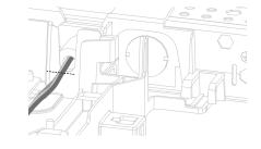
Carefully remove the cord from the product. Set toroid aside to for later use.
