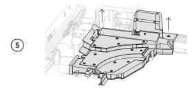
Lift the cover upwards until you are able to pull out towards you to remove.
