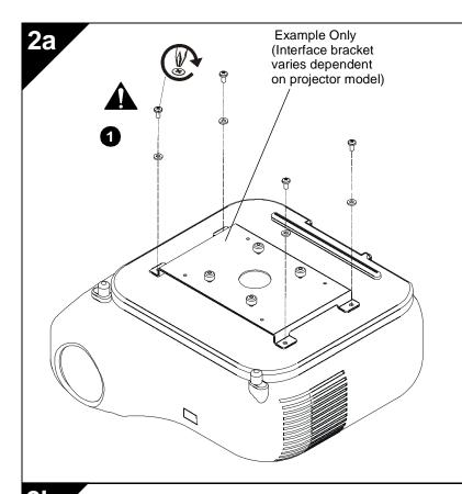
WARNING: IMPROPER INSTALLATION CAN LEAD TO PROJECTOR FALLING RESULTING IN SERIOUS PERSONAL INJURY OR DAMAGE TO EQUIPMENT. DO NOT substitute hardware. Use only the hardware provided by the manufacturer.
