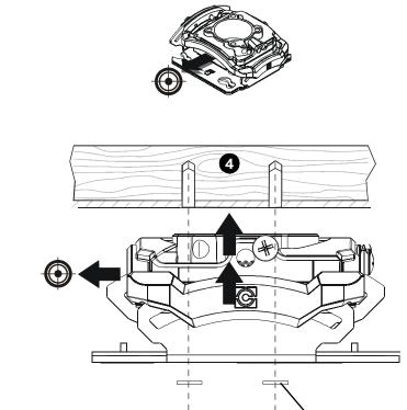
Align four mounting holes in RSM with four pilot holes.
