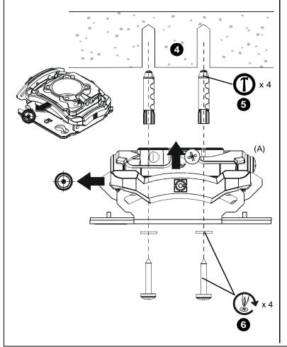
4. Align four mounting holes in RSM with four pilot holes.
