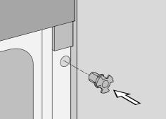
Insert the mounting aid into the hole in the front frame.
