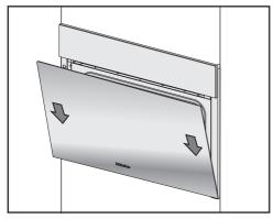
Hold the door securely on both sides and carefully install it back into the hinge retainers.
