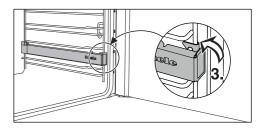
Then secure the FlexiClip telescopic runner to the lower rail of the shelf level (3.).
