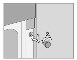
Screw the knurled nut onto the bolt by hand to fix the steam oven in the housing unit.
