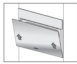
Hold the door on either side and evenly pull diagonally upward from the hinge retainers.
