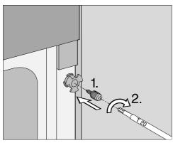
Insert the bolt into the mounting aid and tighten it in the housing unit.
