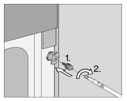
■ Insert the bolt into the mounting aid and tighten it in the housing unit.
