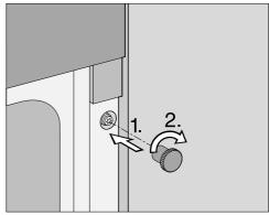
Screw the knurled nut onto the bolt by hand to fix the steam oven in the housing unit.
