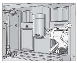
Pull the brew unit to the side ① first and then pull out to the front ③. Tilt the brew unit forward ②.
