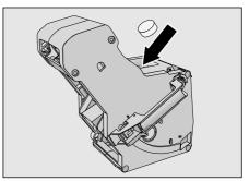
Drop a cleaning tablet into the top of the brew unit (arrow).
