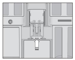
Insert the dispensing unit into the coffee machine and connect the milk pipework.
