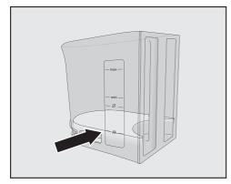
Fill the water container to the //// mark with lukewarm water and stir the solution.
