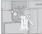
Detach the milk pipework from the dispensing unit ①. Pull the dispensing unit down to remove it 2.
