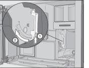
Press the button under the handle of the brew unit ① and, while doing so, turn the handle forward 2.
