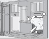
■ Pull the brew unit to the side (1) first and then pull out to the front (2). Tilt the brew unit forward (3).
