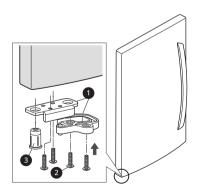
6 Use a ¼ in (6.35 mm) hex socket wrench to loosen the hinge pin **1** and remove. Remove the two allen screw using 5 mm (3/16 in) **2**, the phillip screw **3** and the hinge **4**.
