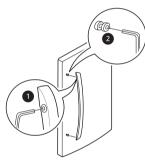
3 Carefully loosen the plug buttons with your fingers. The buttons can be unscrewed with the fingers by rotating them counter-clockwise and continuing until they loosen and fall out The buttons were installed without pressure, and for this reason, they can be unscrewed using your index finger, thumb or both. Install the plug buttons on the left side.
