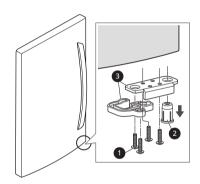
5 Reinstall the hinge pin brackets ①, screws
