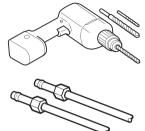
• If your existing copper water line has a flared fitting at the end, purchase an adapter (available at plumbing supply stores) to connect the water line to the refrigerator OR cut off the flared fitting with a tube cutter and then use a compression fitting.
