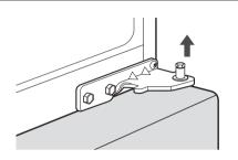
4 Remove the four screws ①, the hinge pin insert ② and the hinge pin brackets ③ from the bottom right side of the door.
