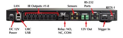
DC 12V Power: Attach the included 12V DC 3.5A power supply here.
