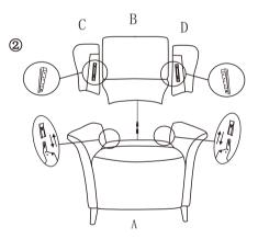
2. Place Bracket into Sleeve and press top of back down firmly to lock your KD back and KD wings in place Connect the connector of back and seat.
