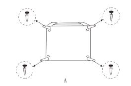
1. Please assemble the legs first before turning over the chair in order to avoid motor broken. Take down the bag from the bottom of the chair, legs are packed inside. Rotate the wood leg with washer and plastic leg clockwise in place.
