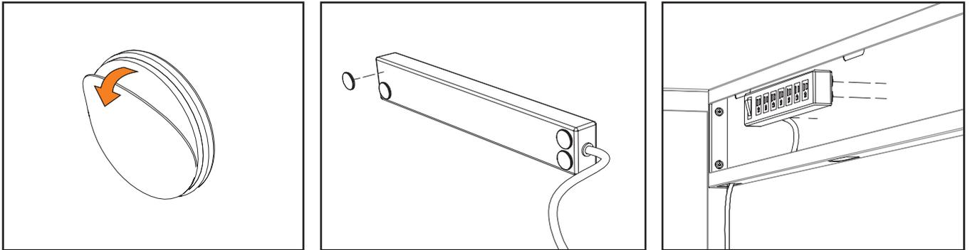
Your Linea Work Desk is equipped with built-in levelers. Dial down one or more levelers (by hand) until you attain a level stance.
