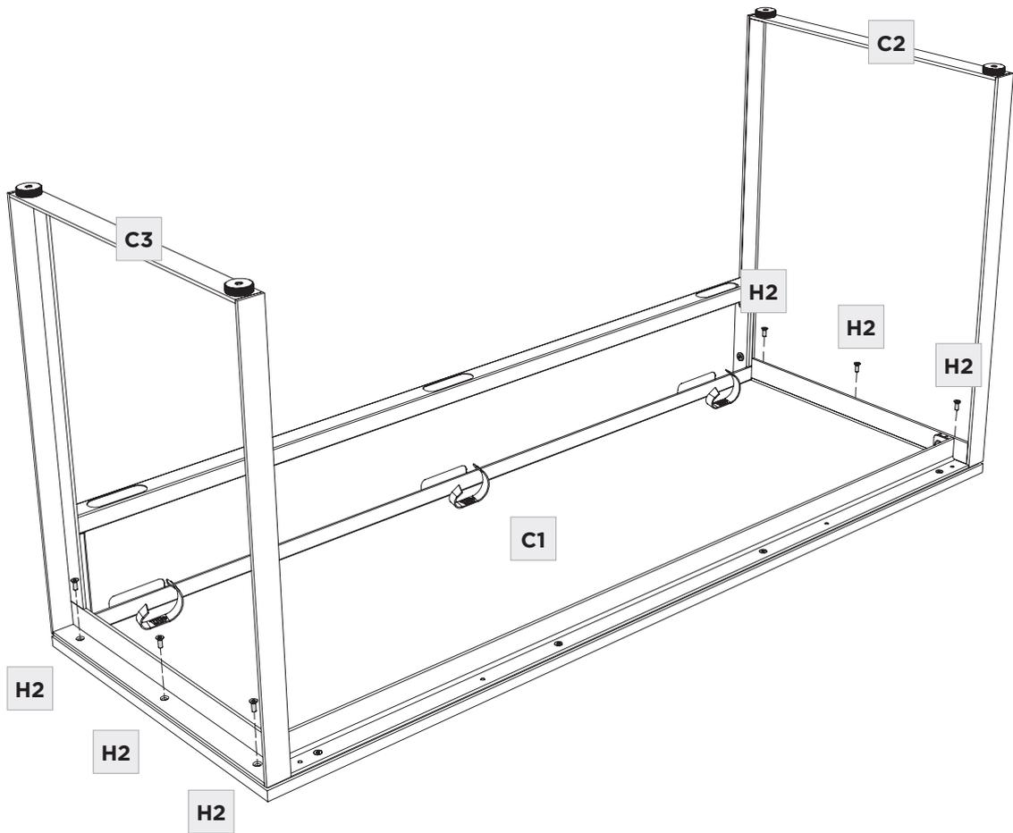
**STEP 4. INSTALL WIRE MANAGEMENT EXTRUSION**
