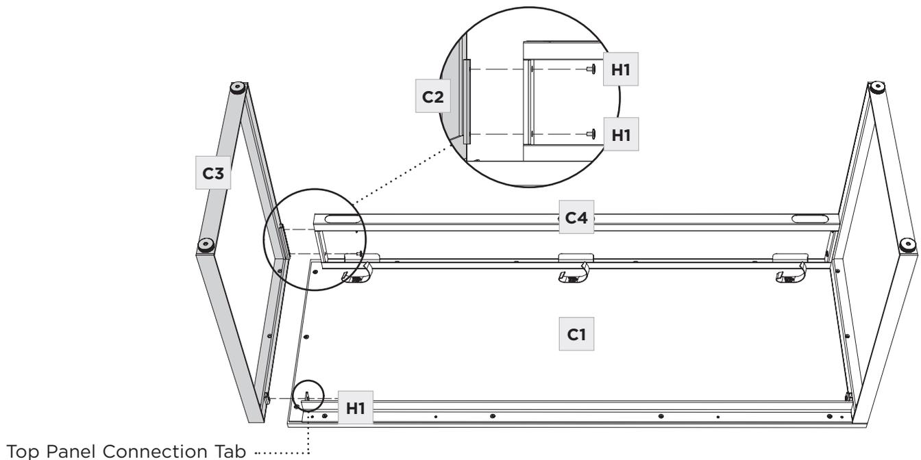
Fasten **(C2)** and **(C3)** Leg Frames to **(C1)** Top Panel using **(H2)** Screws. Tighten all screws connecting **Legs** and **Wire Trough**.
