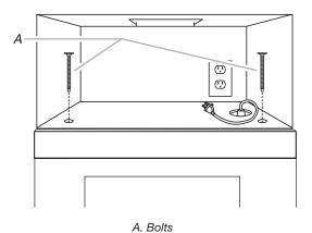
**NOTE:** Avoid damage to the mounting nut, screw the bolts into the mounting nut holes around 15-20 mm by hand first, make sure the bolts thread in properly. Then tighten with tools.
