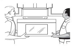
**4.** Using 2 or more people, lift microwave oven and hang it on support tabs at the bottom of mounting plate.
