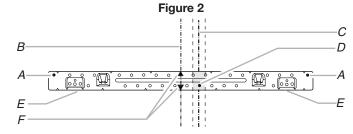
**NOTE:** If wall stud is within 6" (15.2 cm) of the vertical centerline (see the "Mark Rear Wall" section), only recirculation or roof venting installation can be done.
