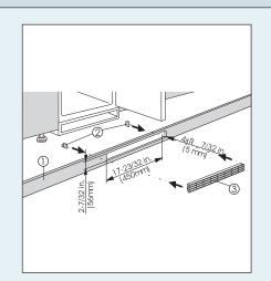
Ventilation through the cabinet base at the bottom can be achieved by installing the provided ventilation grille (3) or via a ventilation opening of at least 31 in.<sup>2</sup> (200 cm<sup>2</sup>).
