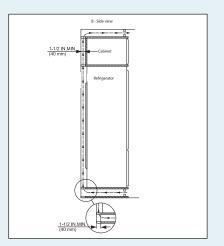
This is a fully integrated refrigerator-freezer which means that it is fully enclosed by a kitchen cabinet. This type of cabinet must be carefully constructed using the correct dimensions and it must provide suitable ventilation to ensure proper appliance operation.
