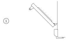
Holding the door at 45°, carefully align the hinge tongues with the hinge slots. Push the door in until you feel the latches slot into position on each side.
