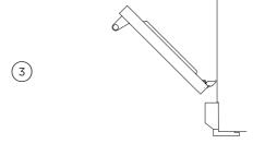
Holding the door on both sides, lift door back up to  $45^{\circ}$  and carefully pull the door out and away from the hinges.
