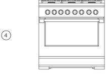
Close the oven door ensuring that when closed, the door is vertical and parallel to any surrounding cabinetry
