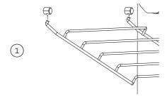
Supporting the side rack from underneath, hold it almost horizontally and place the prongs into the mounting slots.
