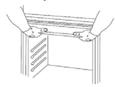
2. Feed the flexible electrical supply conduit from the oven to the junction box.
