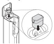
Press the battery down into the compartment.
