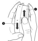
**10** Insert the clean, dry pre-filter and rotate the exhaust filter to the locked position 6 to reassemble it on the product body.
