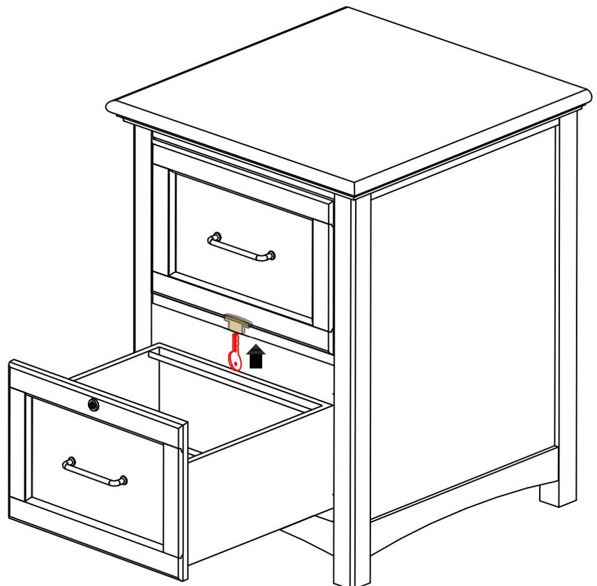
**NOTE:** The T-Lock is located in the center of the wood crossbar.
