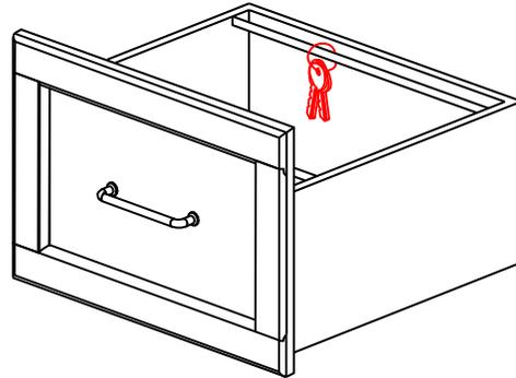
The T-Lock affects both the drawer that it's attached to and the drawer directly above it.
