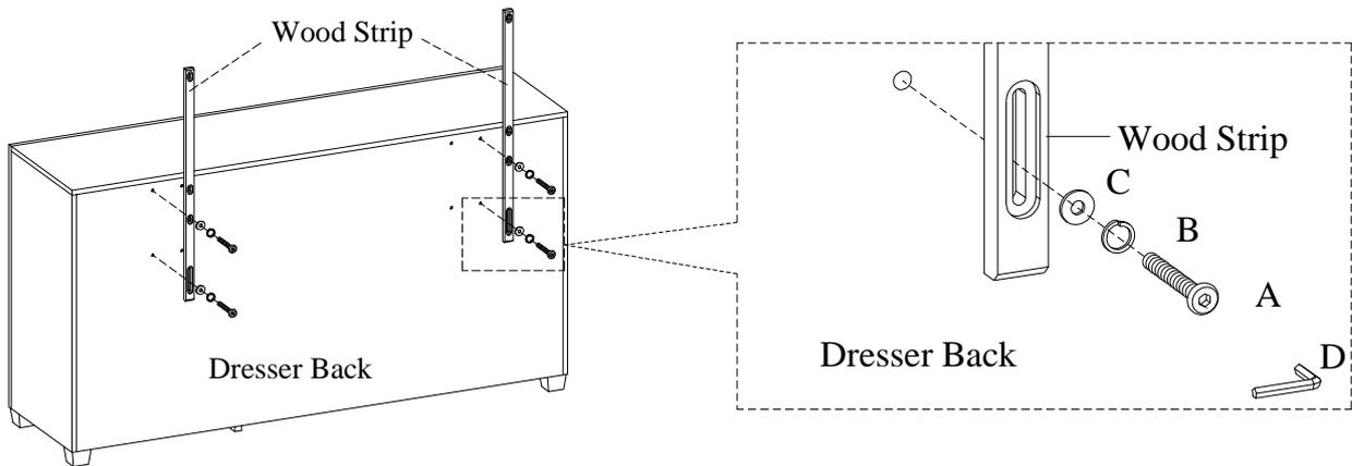
STEP 2: Attach the wood strip to the mirror by using 4 bolts(A), lock washers(B), and flat washers(C). Tighten all bolts on dresser and mirror with Allen wrench.
