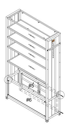
1) Align back frame (#6) to the unit, then secure by using bolts (#A).
