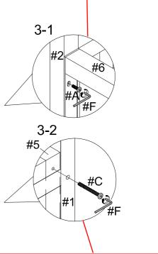
2) Align front frame (#5) to the unit, then secure by using bolts (#C).
