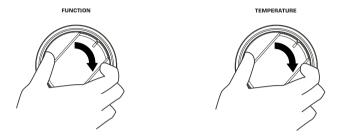
① Select the oven function and temperature. Preheat the oven if appropriate. Remember ROAST and CONV BROIL do not require preheating.
