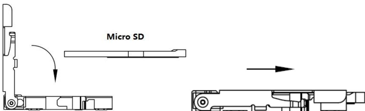
Figure 2-4 Micro SD Card installation illustration 2
