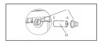
9. Open the door, place the 20-pound cylinder into the main body and tighten it as shown on the right, so the gas cylinder cannot move and fall down, close the door ,put the Burner Cover on the fire pit table top,then cover the fire pit with PVC cover (L)when not in use to protect it from the elements or when fire pit is cool COMPLETELY after the use.
