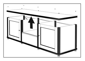
**3**Insert speaker by sliding down posts level, with flat nuts loosely installed to post slots.
