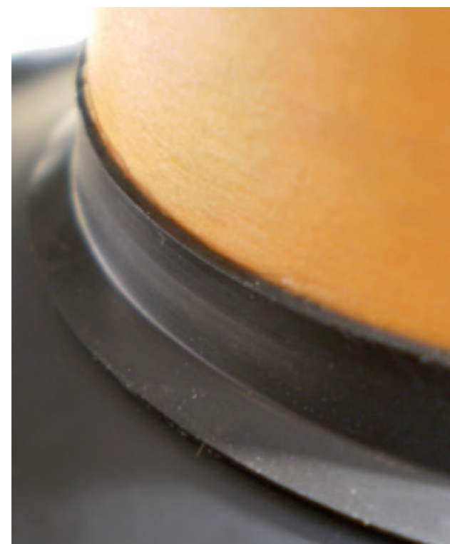
Figure 18 lossy interface between voice coil and midrange cone
