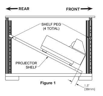
**3.** Continuing holding the back end of shelf, while a 2nd person lifts the shelf up and slightly forward until the projetor lens housing goes through the opening in the top and the shelf can be rested on the front shelf peg as shown in figure 2.
