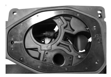
With a reciprocating air saw or preferred cutting device, carefully cut following markings from Step 5. Be carefull on cutting depth. Failure to do so will result in cutting through the soundbar.
