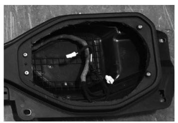
7 Fill the right and left speaker cavities using (1) of the supplied polyfil sheets per cavity.
