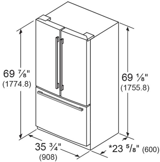
\* Add 1 3/8" (35) in the back measurements for proper ventilation
