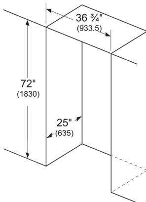
Leave 2" (50.8) gap at the top and 1 3/8" (34.9) behind the refrigerator for proper ventilation.
