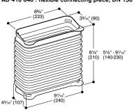
AD 851 041: Connecting piece VL for extension with flat duct DN150 for extra deep countertop
