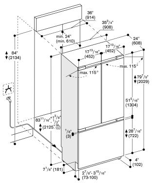
The door face dimensions are designed for a maximum gap of 1/6" (3 mm).
