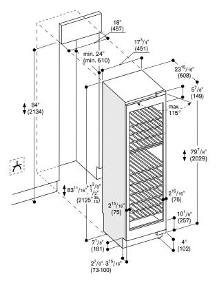
The door face dimensions are designed for a maximum gap of 1/6" (3 mm).
